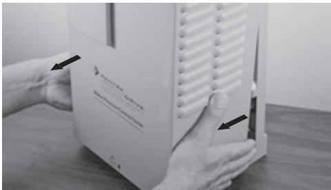
Figure 5 - Pull out bottom of cover
